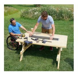
Now, utilise the table cut outs, plus some of the extra timber, to build a support for the grill box. This will also protect peoples' legs from heat. Clamp the wood in place and secure with screws.
