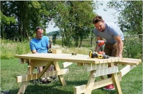
Once the seat supports have been extended and a brace bar installed to hold them at table height, drill holes for inserting the M8 bolts, at both levels. These will secure the extensions you have made, when being used as seats, or table extensions.
