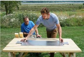
Use the clamps and the wood you cut out of the table top, to hold the steel against the table edge. This will give you enough resistance to bend the steel into a box shape. The hammer allows you to form a crisp edge.
